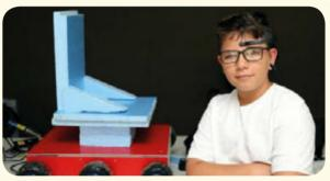
Efe İnan lives in Antalya. He developed a portable wheel chair for paraplegic people. This wheel chair moves with mental capacity. It has a headdress and it gets signals from certain neurones. So, the signals drive the wheel chair back and forth. This machine has 6 motors and a battery. With this project, paraplegic people spend their lives without needing any help. In the future, Efe will develop his invention and this invention will be a great hope for thousands of paraplegic people.
